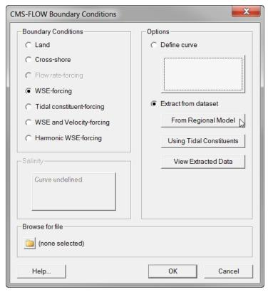
Figure 2-54. CMS-Flow Boundary Conditions window in SMS 11.1 with an WSE boundary condition.
