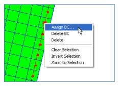
Figure 2-40. Opening the CMS-Flow Boundary Conditions window by left clicking.
