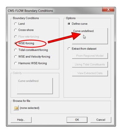
Figure 2-47. Defining the single water surface elevation curve.
