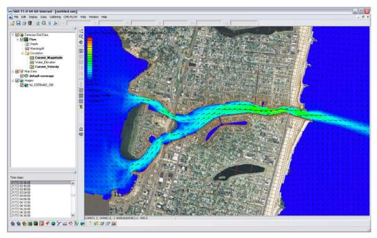
Figure 7-6. Vectors and color contours set for displaying current magnitude (color) and direction (vectors). Note that the vectors are slightly scaled on this setting to reflect magnitude.
