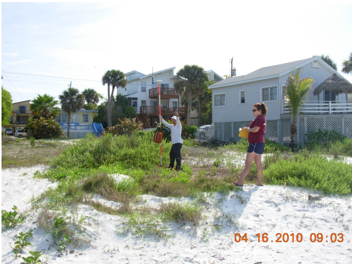
Figure 8. Temporary Benchmark Establishment. At each line, two stakes were placed so that the same line could be reoccupied and surveyed again.
