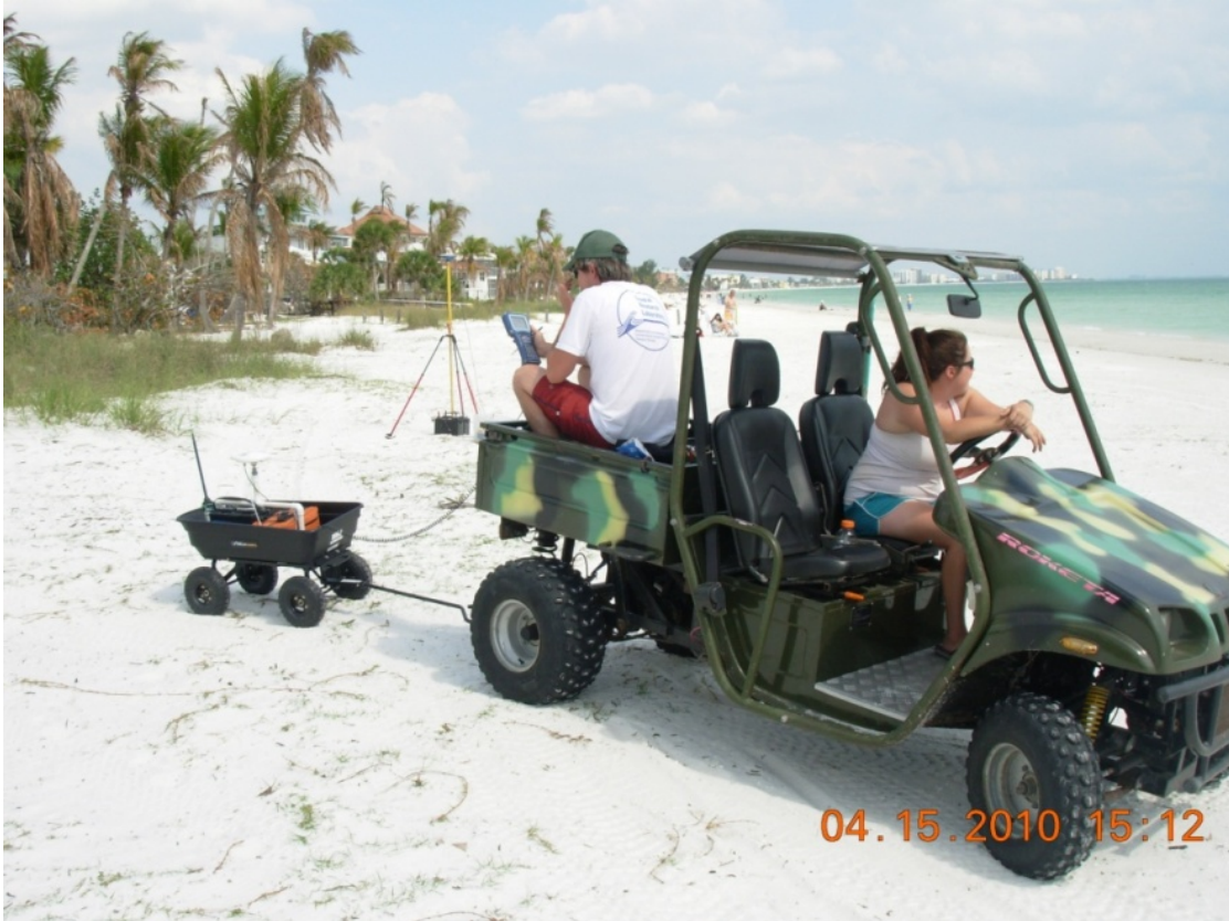
Figure 9. Shoreline Survey Using an ATV and a Cart. A small cart was towed by an ATV for shoreline surveys.
