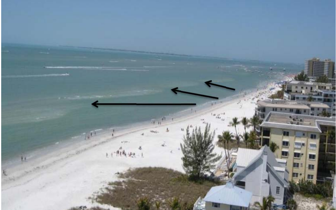
Figure 38. Longshore Variations in the Berm (March 2010). Notice that the gaps in the berm are at an oblique angle to the shoreline.
