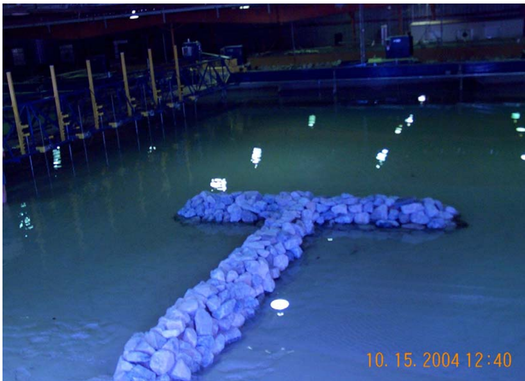
Figure 114. T-groin structure in filled LSTF at operating water level.
