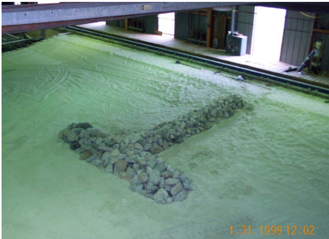
Figure 113. Completed T-groin structure in LSTF model beach.
