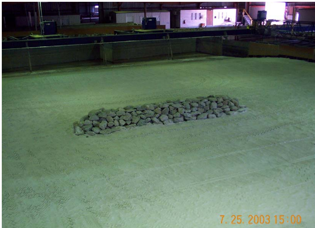
Figure 30. Completed breakwater structure in LSTF model beach.
