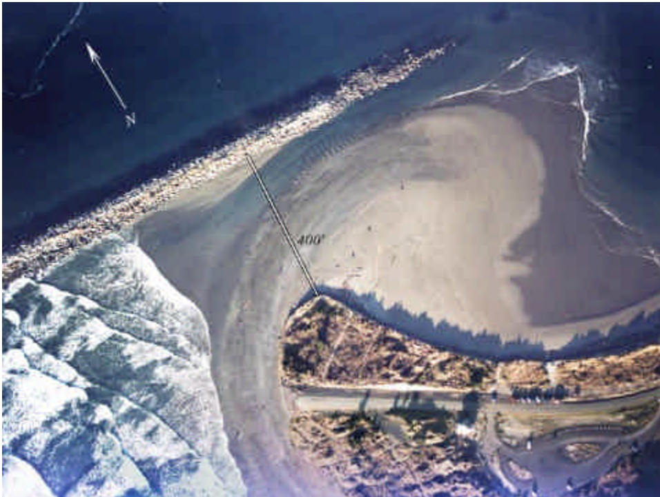
Figure 2-1. Breached area at South Jetty Grays Harbor, 1994
