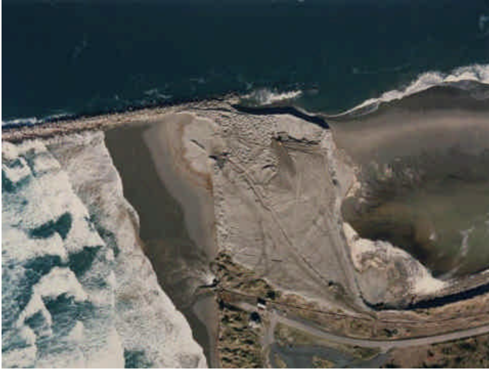
Figure 2-2. 2 November 1994 during placement of breach fill
