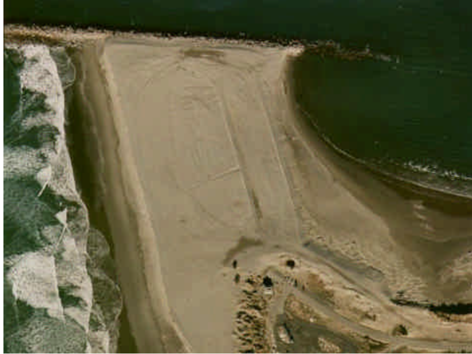
Figure 2-4. 1 February 1996 approximately 13 months following placement of 600,000 cu yd of dredged sand in the breach
