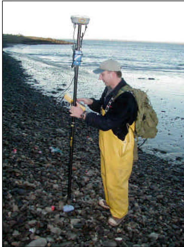
Figure B-3. Surveying the initial placement of tracer particles with an RTK-GPS
