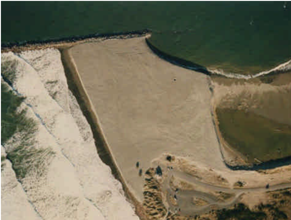
Figure 2-3. 3 January 1995 following placement of 600,000 cu yd of dredged sand in the breach
