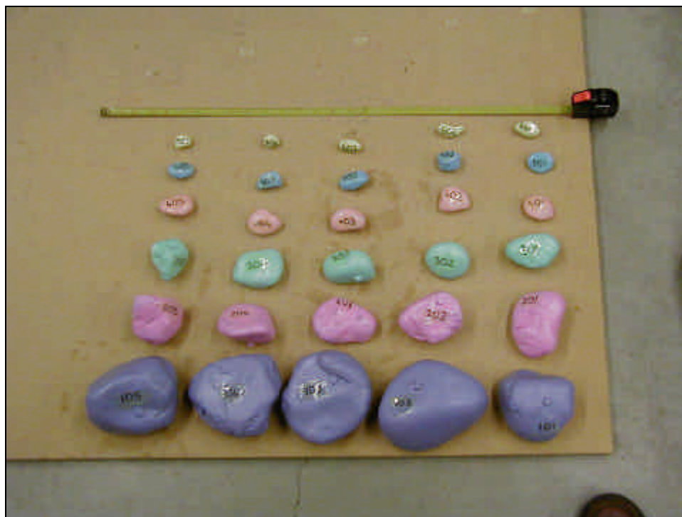
Figure B-2. Photo showing magnetized tracer particles prior to deployment
