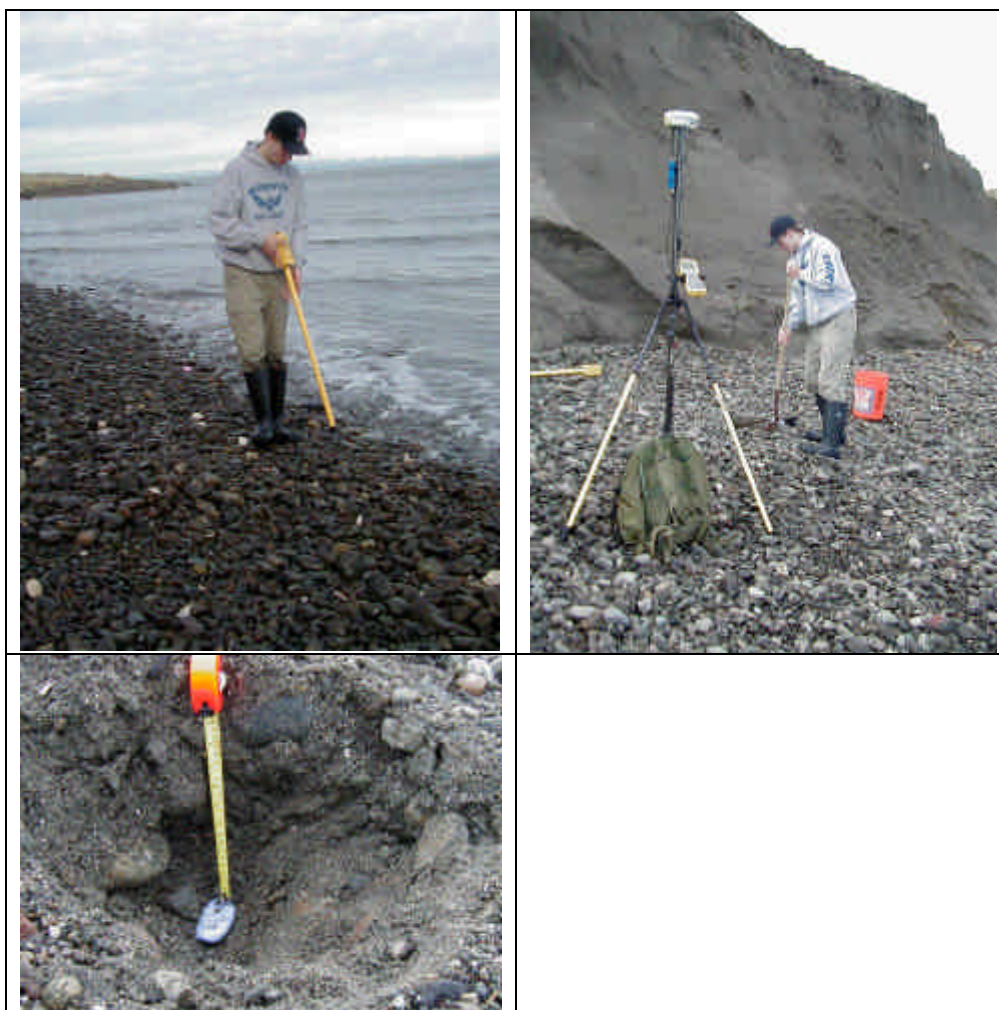
Figure B-4. Relocation of tracer particles using a magnetic detector, RTK-GPS survey system. Depth below the sand surface was also recorded in cases where particles were buried
