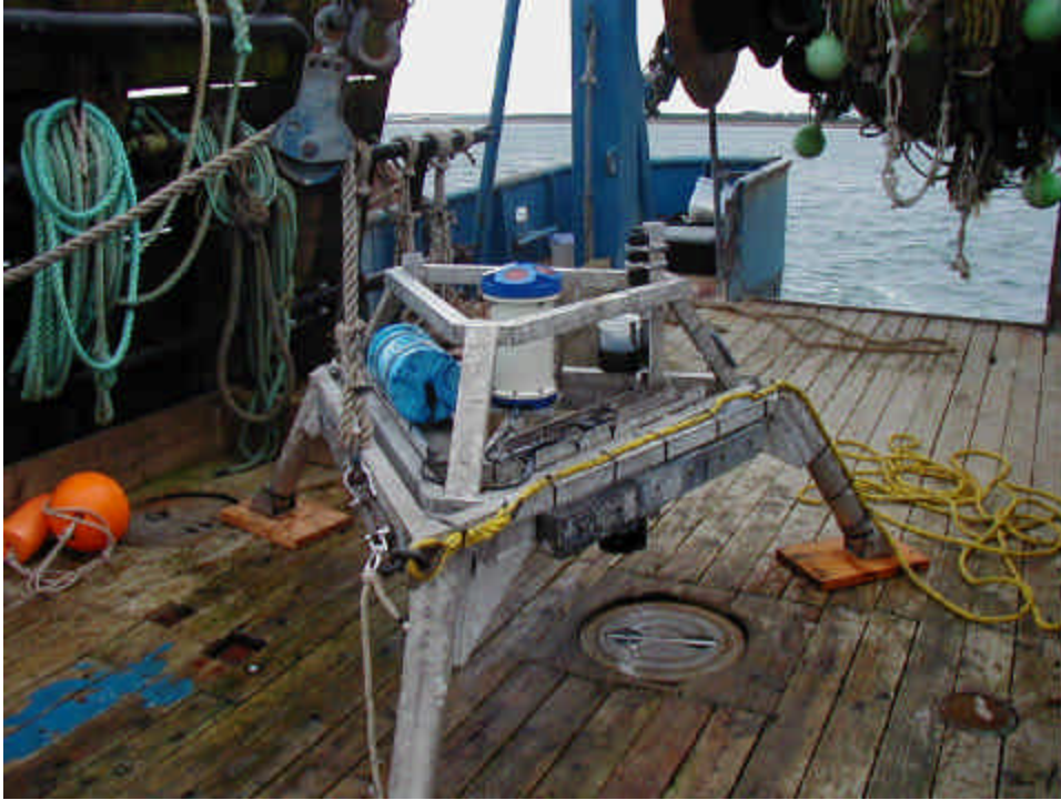
Figure A-2. HM1 tripod instrument platform with ADCP prior to deployment
