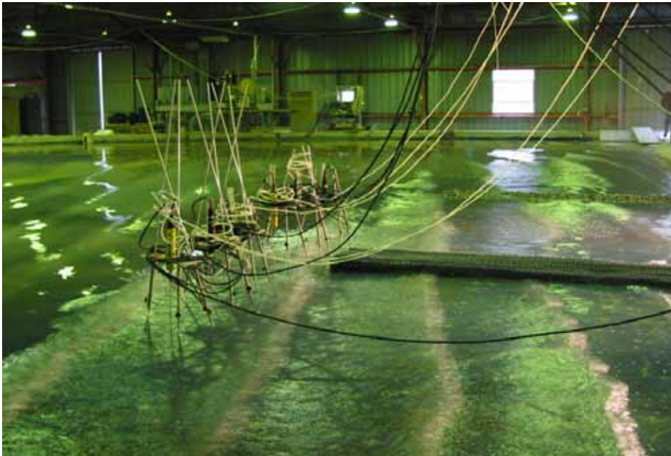
Figure 12. Current meters seaward of jetty
