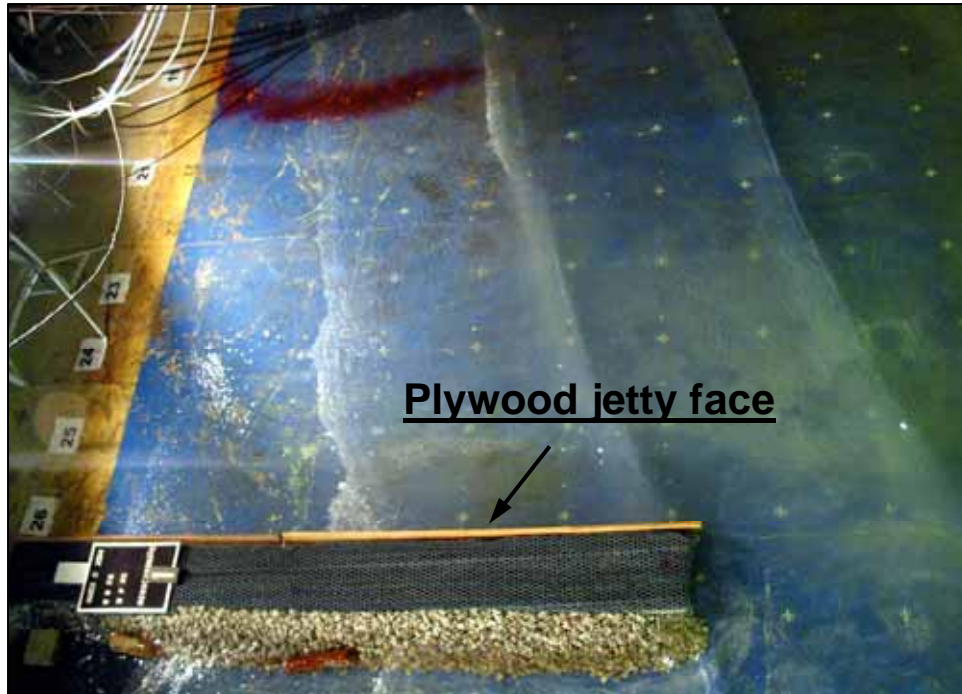
Figure 10. Plywood reflecting jetty face
